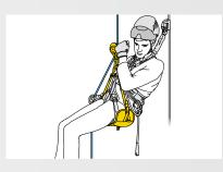
Self-braking descenders are versatile and can be used for both descents and short rope ascents.
