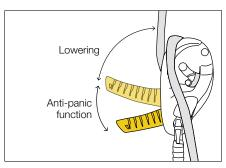
Designed for work at height, rope access, and technical rescue and evacuation, these devices are equipped with an anti-panic function and an anti-error catch, limiting the risk of an accident due to user error. They are also compatible with auxiliary brakes, in order to increase the braking friction for descents with heavy loads.
