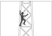
The ABSORBICA-Y lanyards with two arms allow for continuous protection, by successively detaching and re-attaching the two arms.
