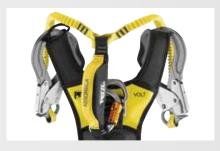
The harnesses have a stowage system for the MGO connectors on fall arrest lanyards on each shoulder strap. In case of a fall, the system releases the MGO connectors and allows the absorber to be deployed.
