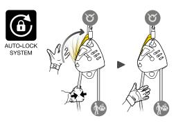
Hauling is possible at any time, without manipulating the handle.
