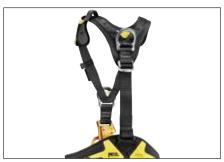
ASTRO BOD FAST full-body harnesses are equipped with a dorsal attachment point for attaching a fall arrest system. In case of a fall on this attachment point, a shorter adjustment of the length between the waistbelt and the leg loops means the load is taken up on the leg loops, allowing the user to remain suspended longer while awaiting rescue.
