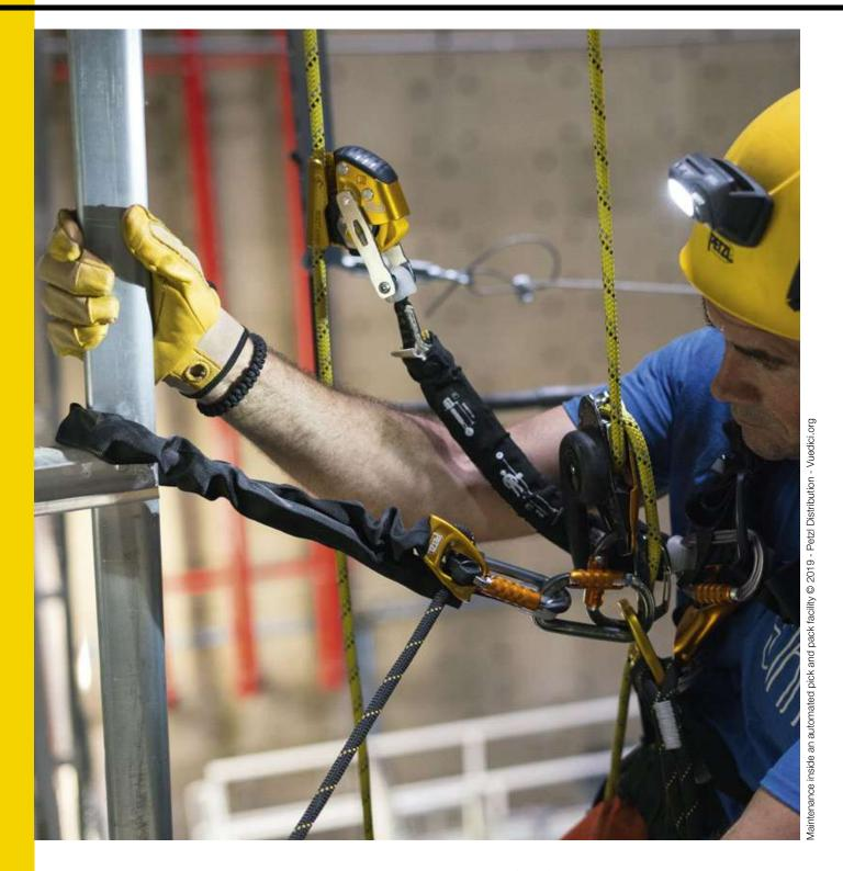
Depending on the model, the ends of Petzl lanyards are equipped with plastic sheaths, or with STRINGs. These items help keep the connector positioned on the major axis, and facilitate clipping. They also protect the ends from abrasion due to repeated rubbing.
