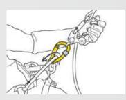
The ROLLCLIP Z pulley can be used for tree care to attach the ZIGZAG descender to the attachment bridge on the SEQUOIA harness, for improved lateral mobility.
