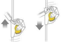
The ASAP and ASAP LOCK mobile fall arresters follow the worker in all his/her movements, without the need for any manual operation. S/he can therefore focus completely on the task.
