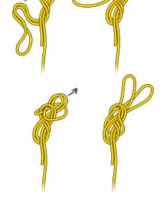
Special case: isolate a section of damaged rope with a butterfly knot.
