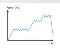
In case of a fall, the tearing of the energy absorber webbing limits the impact force on the user. The lanyards are designed for users who weigh between 50 and 130 kg. The progressive tearing of the webbing reduces the deceleration on lightweight users.
