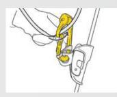
The ROLLCLIP A pulley can be used as a directional point when combined with the RESCUCENDER rope clamp.
