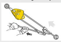
The integrated progress-capture pulley with very large diameter sheave mounted on sealed ball bearings rotates in only one direction for excellent hauling efficiency. The lower connection point can be used to create different types of hauling systems.
