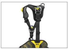
The AVAO BOD and AVAO BOD FAST full-body harnesses are equipped with a dorsal attachment point for connecting a fall arrest system. In case of a fall on this attachment point, a shorter adjustment of the length between the waistbelt and the leg loops means the load is taken up on the leg loops, allowing the user to remain suspended longer while awaiting rescue.
